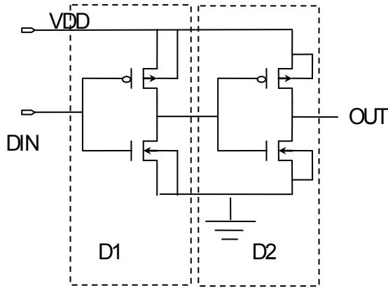
Fig.1. Deviding the buffer into two DCCC ( $D1, D2$ )
