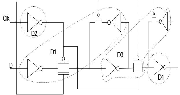
Fig.3. DCCC decomposition of CMOS trigger
