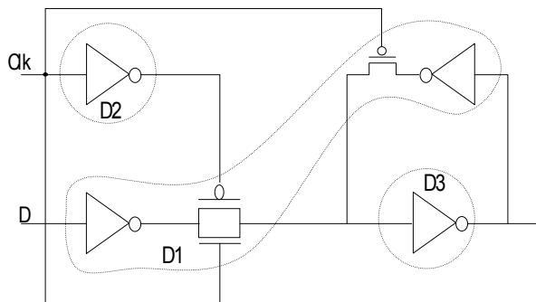
Fig.2. DCCC decomposition of CMOS switch ( $D1, D2, D3$ )
